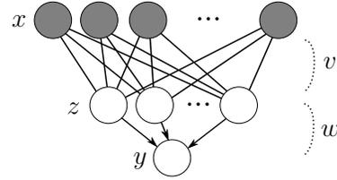
Figure 1: The latent variable model:  $\mathbf{x}, \mathbf{z}, y$  are random variables, dependencies between  $\mathbf{x}$  and  $\mathbf{z}$  are parameterized by matrix  $\mathbf{v}$ , and dependencies between  $\mathbf{z}$  and  $y$  - by vector  $\mathbf{w}$ .
